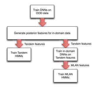
Figure 1: Multi-Level Adaptive Network (MLAN) architecture
